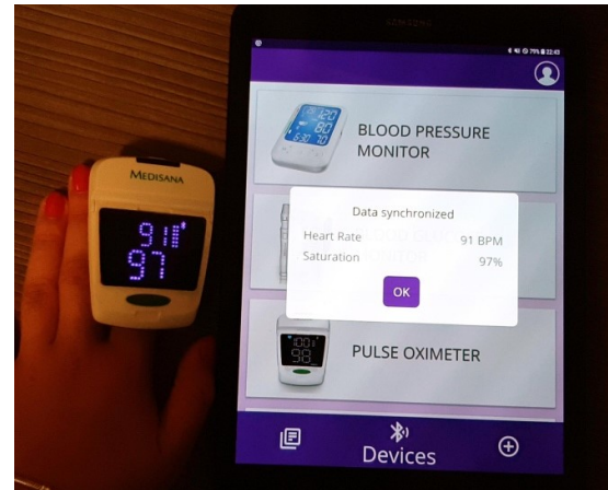
Figure 2. Synchronizing data between medical device and mobile app
